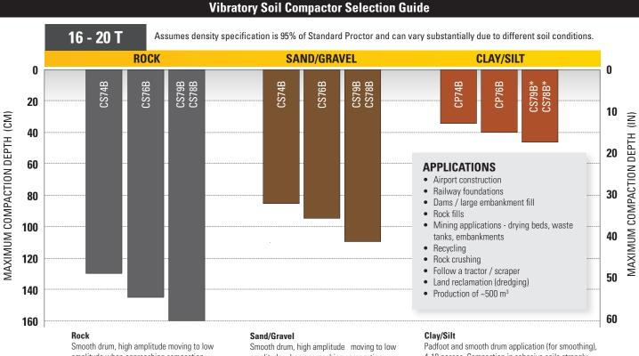
Smooth drum, high amplitude moving to low amplitude when approaching compaction, 4-8 passes
